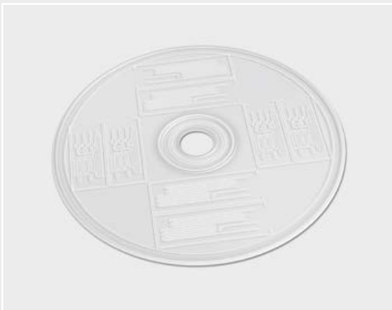
The transparent microfluidic wafer was welded with the new ClearJoining technology
